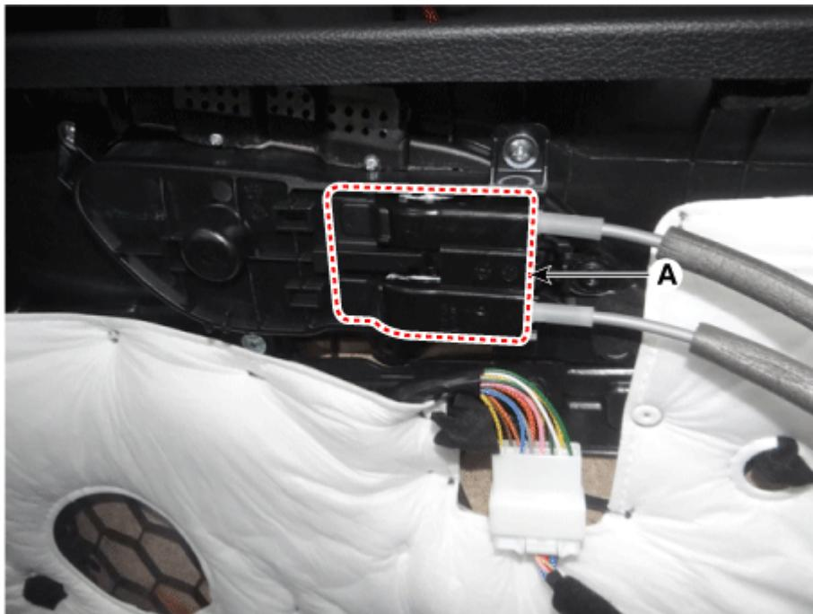
5. Disconnect the power window switch connector (A) and rear door tweeter speaker (B).
